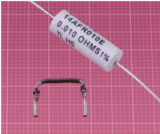
Figure 30-7 Two styles of current resistors rated for 0.01 ohms. Bottom left: A plug-in version from TT Electronics, rated 1W and 5%. Top right: Ohmite, 4W, 1%. The background grid is in millimeters.
