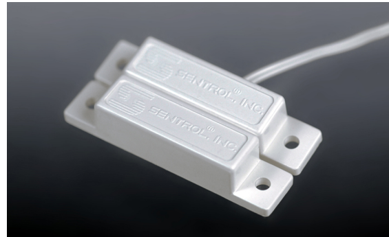
Figure 3-12 A typical alarm sensor to detect the opening of a door or window. The nearer module contains a magnet, while the module behind it contains a reed switch.
