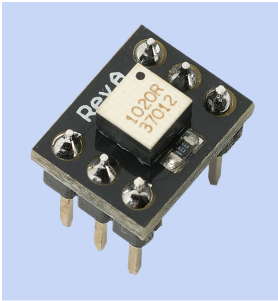
Figure 8-9 A 2-axis tilt sensor mounted on a breakout board available from Parallax.
