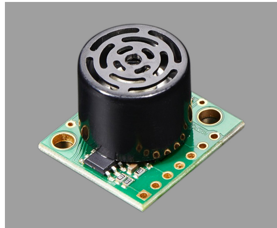
Figure 5-3 The MaxSonar MB1003 can detect large solid objects as far away as 5 meters. Photo derived from an image by Adafruit.
